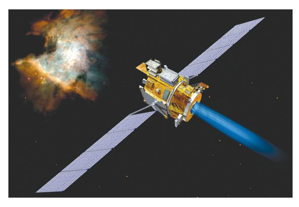
electric charge by rubbing it on wool. The xenon ions shoot past the grids at speeds of more than 88,000 mph (146,000 kilometers), continuing out the back of the engine and into space. These exiting ions produce the thrust that propels the spacecraft.
