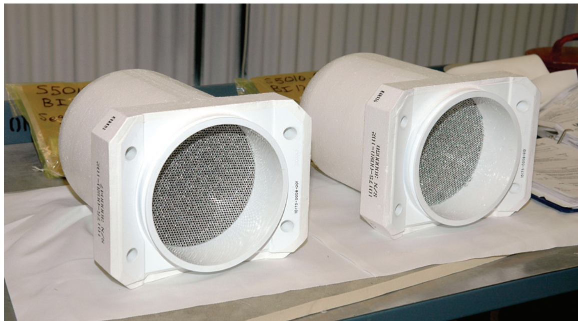
These two bolt catchers are ready for installation on orbiter Discovery's External Tank.
