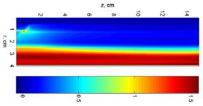
Rotational Mach number the pellet ablation flow demonstrating supersonic rotation of the channel, the most likely cause of striation instabilities.
