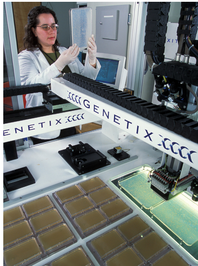
Technician Sarah Batt uses a robot to pick yeast colonies and transfer them onto starch plates, where they'll be screened for desirable enzyme production.
