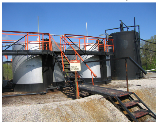
Tank farm where oil/water mixtures from multiple wells are collected and separated. Faculty hatches on the tanks have been shown to be a significant source of hydrogen sulfide release.
