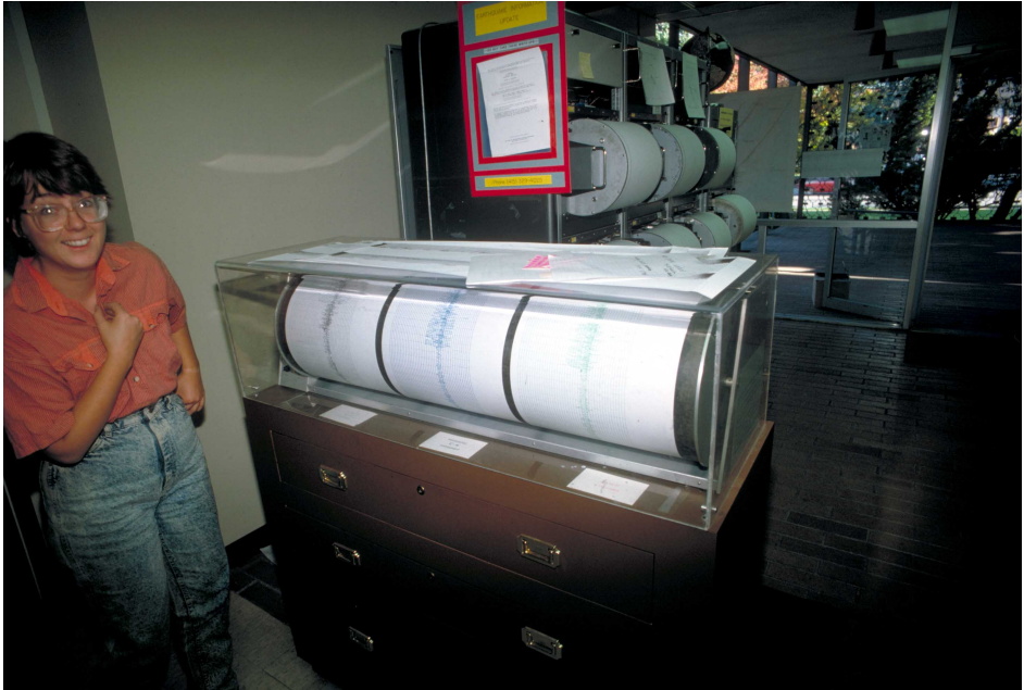
41. Seismographs at the U.S. Geological Survey record (1) north-south horizontal, (2) east-west horizontal, and (3) vertical components of the earthquake. [J.K. Nakata, U.S. Geological Survey]
