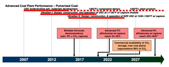
\*for bituminous coal; equally advanced PC plants firing subbituminous coal and lignite will have efficiencies two to four percentage points lower due to higher moisture and ash contents
