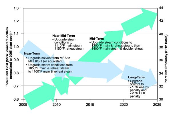
Figure 7 – RD&D path for capital cost reduction (falling arrows) and efficiency improvement (rising arrows) for PC power plants with 90%  $CO_2$  capture
