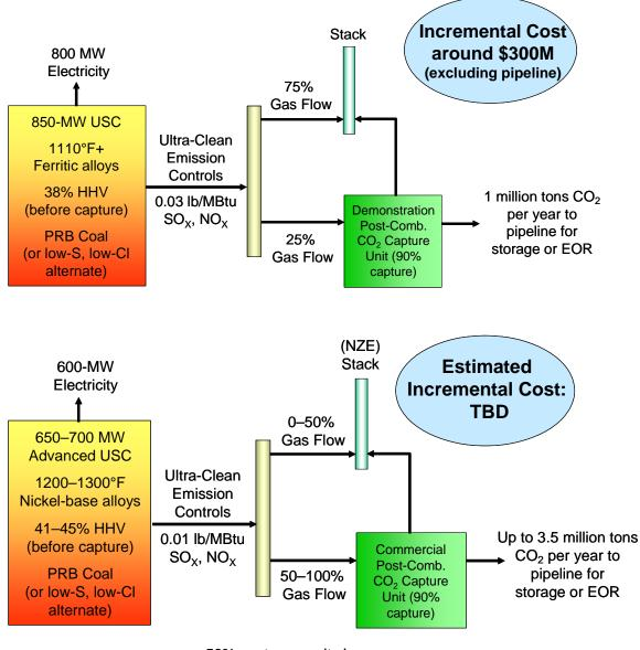
50% capture results in CO<sub>2</sub> emissions of ~900 lb/MWh
