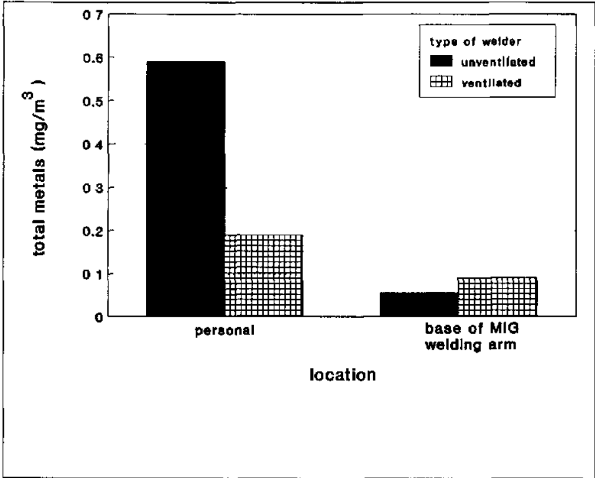
Figure 5 The use of a ventilated MIG welder reduces the workers exposure to metal aerosols inspite of a concentration increase at the area sampling location
