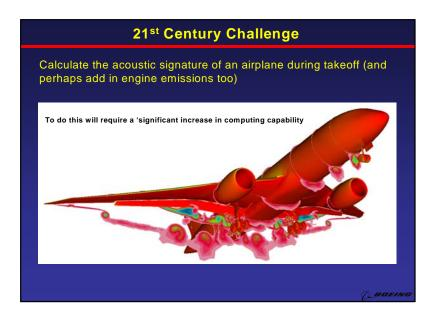
An even greater challenge lies in the area of acoustics. Today laboratory and/or flight tests must be conducted to determine the acceptability of candidate airplane configurations to meet community noise requirements. In the future we hope to do all the simulations within the computer.
