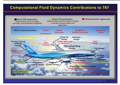
One of the best utilizations of High-Performance Computing is in the development of computational fluid dynamics (CFD). While CFD has been in use at Boeing for 30 years, the most extensive application has been on our newest commercial aircraft, the 787 Dreamliner. The use of CFD tools has allowed Boeing engineers to address a wide range of design challenges, including traditional wing design, the even distribution of cabin air and reduction in overall airplane noise.
