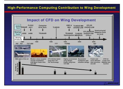
Another example of the benefit of High-Performance Computing and improved computational capability has been in our wing development over the last 25 years. In 1980, Boeing tested 77 wings in wind tunnels to arrive at the final configuration of the 767. Just 25 years later, we built and tested 11 wings for the 787 -- a reduction of over 80%. Those 11 wings took less people to design, less time to design, and the wind tunnel results matched the CFD predictions.
