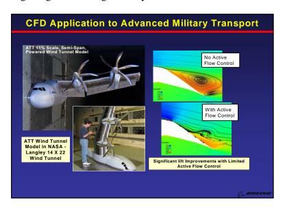
The chart above shows another wing design application which resulted in a configuration that could not have been designed without CFD design tools and High Performance Computing. The Air Force has a requirement for a battlefield delivery transport. It must operate out of unimproved, very short runways -- runways shorter than C-17s can use today. Meeting these
