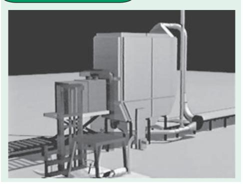
The closed rotary drum system uses less than one-fifth as much energy, requires minimal use of pollution abatement equipment, and allows a retrofit payback period of less than two months.
