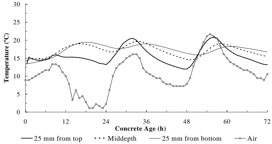
Figure 196. Measured concrete and air temperatures for Minnesota, Slab 1.
