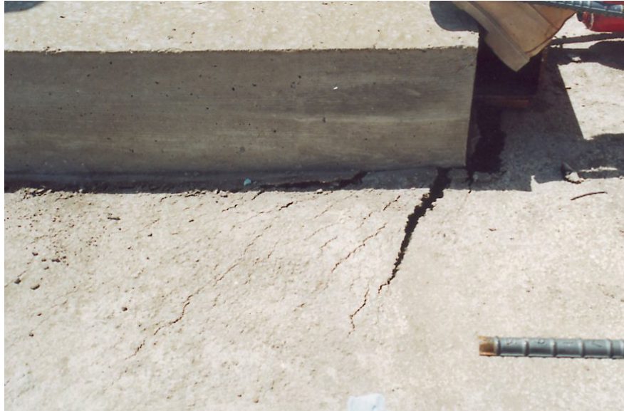
Figure 89. Shear failure as a result of pushoff test.
