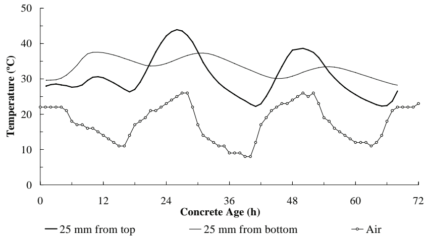
Figure 224. Measured concrete and air temperatures for North Carolina, Slab 2.
