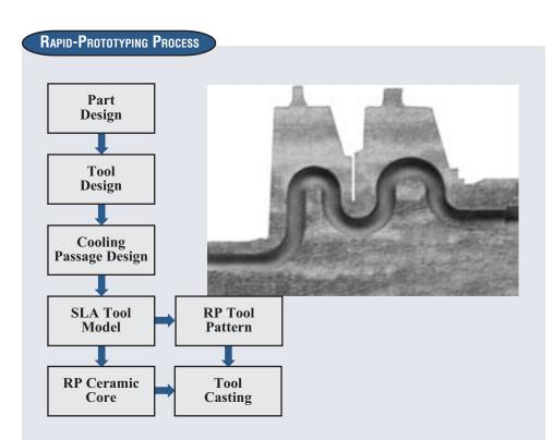
The rapid-prototyping (RP) process provides a more efficient means of reducing cycle times while increasing production rates, which leads to lower energy use and increased profitability for manufacturers. Stereolithography (SLA) will be used to produce patterns of the tool halves with the cooling passages as holes in the pattern.
