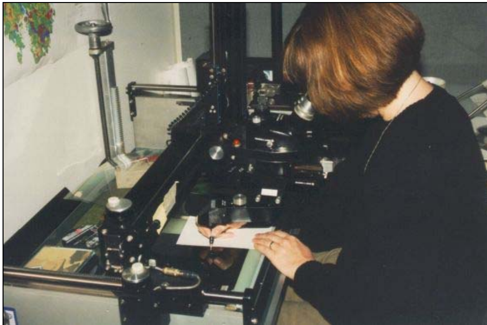
Figure 11. Bausch and Lomb Zoom 240 stereoscope over a Richards MIM2 light table.
