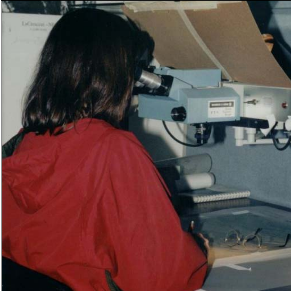
Figure 12. Transferring photointerpreted data to base maps using a zoom transfer scope.
