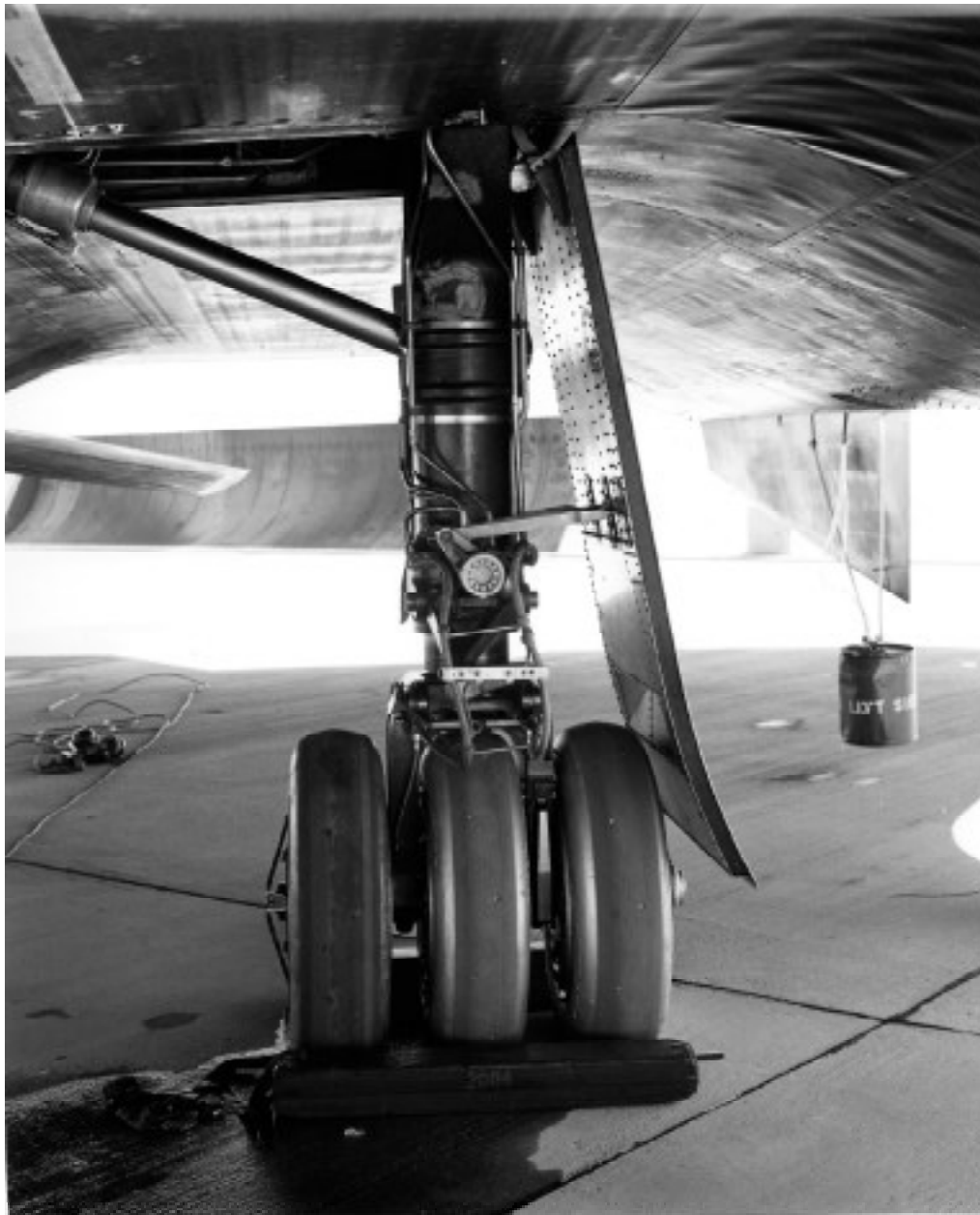
The YF-12A main landing gear included three nitrogen-filled 32-ply tires. They were coated with a thin film of aluminum to reflect heat while retracted. (NASA photo E71-22968)
