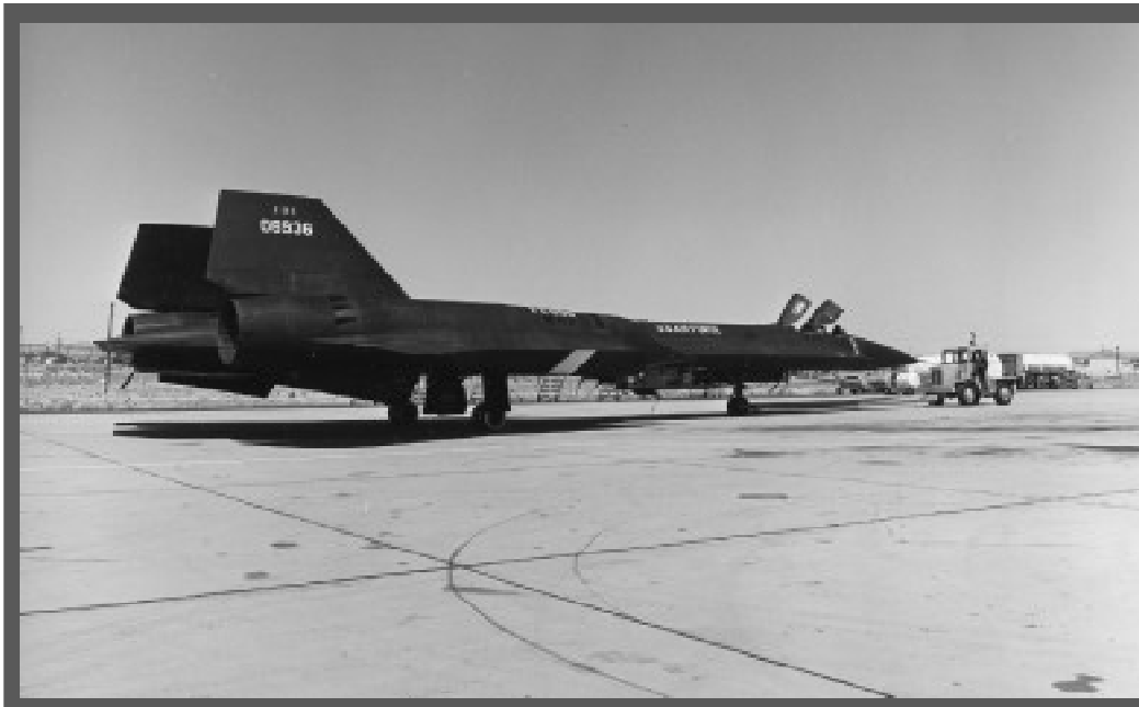
YF-12A (USAF serial number 60-6936) joined the program in 1970 as the primary USAF test aircraft. White markings near the nose commemorate world speed and altitude records achieved by this aircraft on 1 May 1965. (NASA photo EC70-22047)
