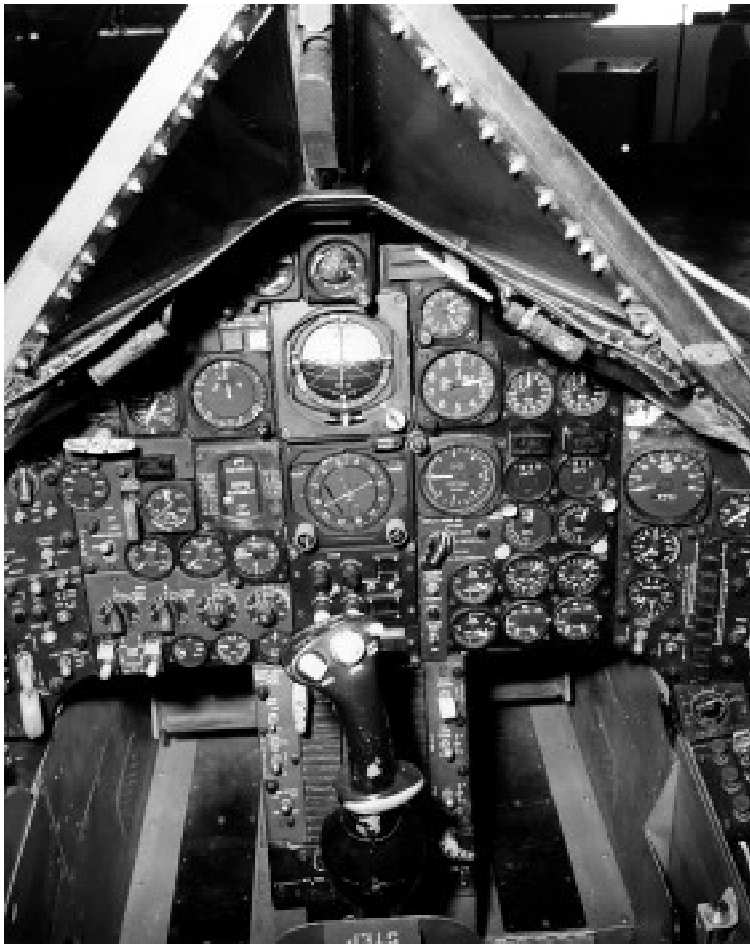
The YF-12C (SR-71A) cockpit. The altimeter and airspeed indicators have been merged into the triple display indicator, below and to the left of the attitude indicator. (NASA photo E72-25349)
