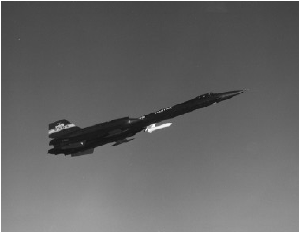
The YF-12A climbs to altitude with the Coldwall heat transfer experiment pod mounted beneath the fuselage. After the aircraft attained Mach 3, the white insulation covering the pod was pyrotechnically removed to expose the nitrogen-cooled stainless steel tube to aerodynamic heating. (NASA photo EC75-4765)
