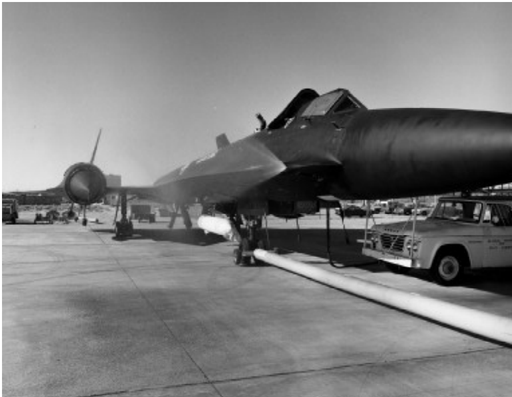
The YF-12A was equipped with a water spray nozzle on the forward fuselage for flow visualization. The system underwent ground tests prior to flight in 1976. Note the Coldwall pod attached on the lower fuselage. (NASA photo E76-31090)
