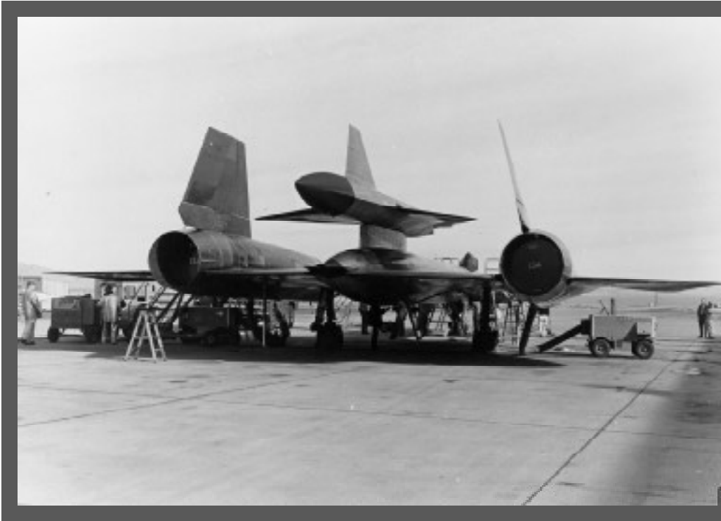
The M-21 variant of the Blackbird carried a D-21 drone on a dorsal pylon. Captive carry tests began in December 1964 and flight tests occurred in 1966. In 1971, NASA pursued the idea of launching a hypersonic test vehicle in a similar manner. (Lockheed photo)
