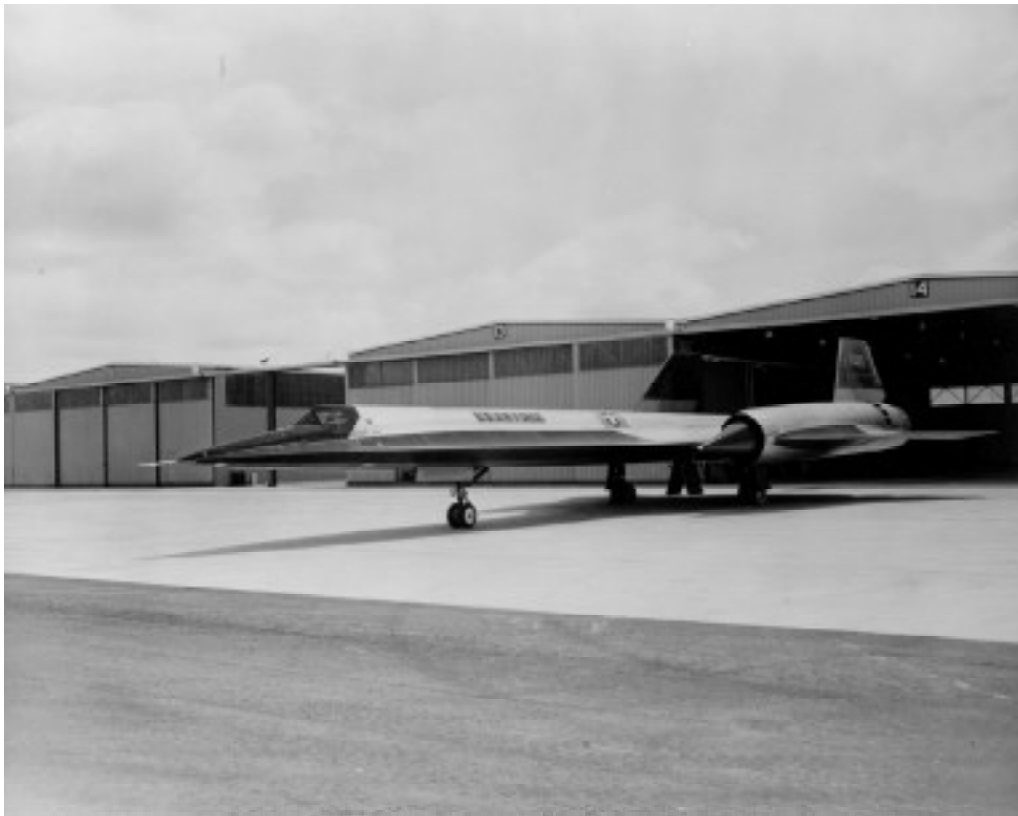
First of the Blackbirds to fly, the A-12 (code-named OXCART) was capable of speeds in excess of Mach 3. The Central Intelligence Agency (CIA) operated the aircraft exclusively from 1962 to 1968. (Lockheed photo)
