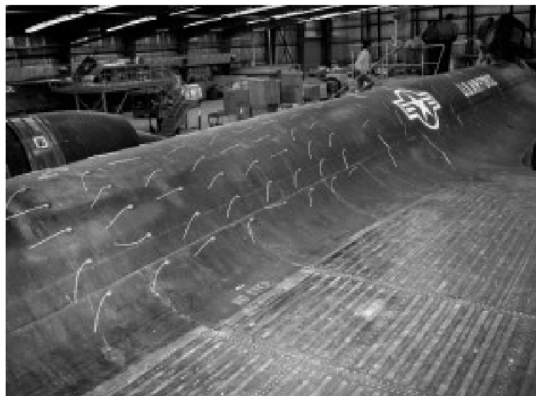
NASA technicians glued tufts to the fuselage of the YF-12A for surface flow visualization studies related to the aft-facing step experiment. (NASA photo E76-31377)
