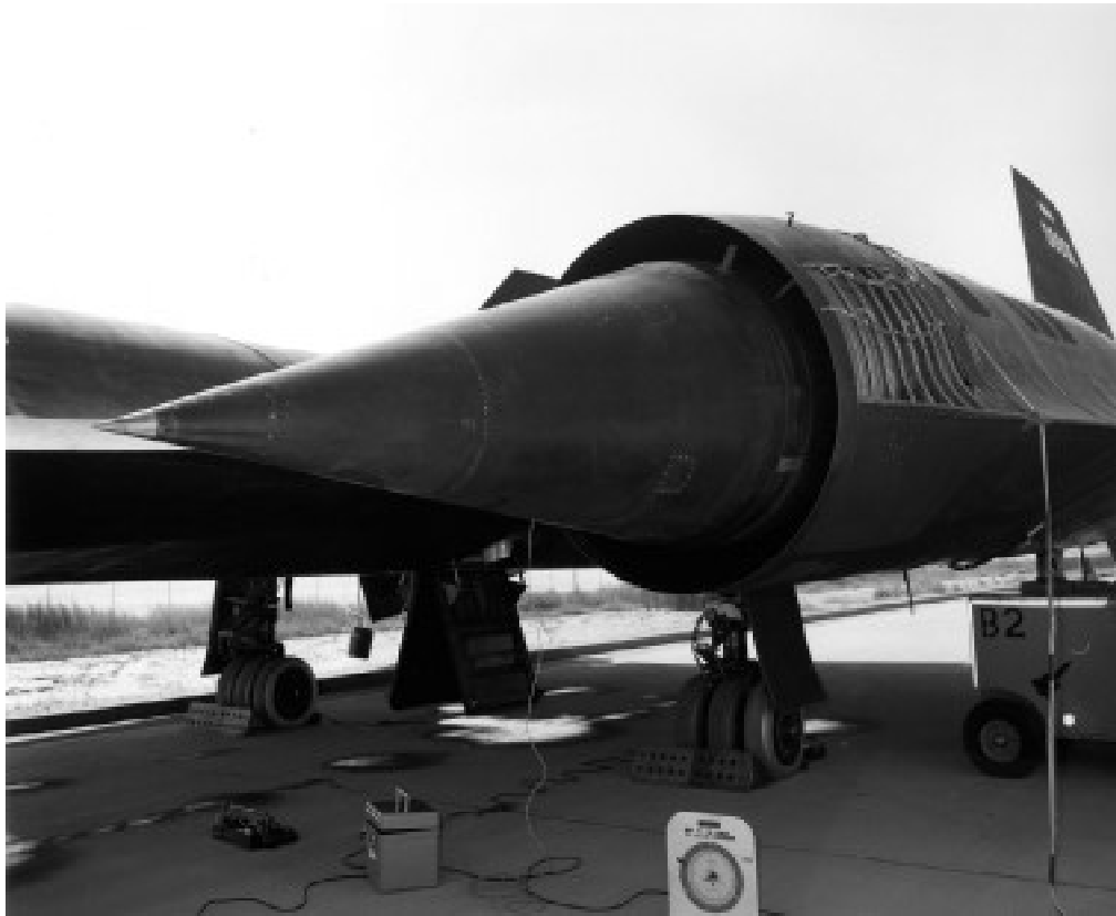
A movable cone, or spike, transitioned forward and aft to control the position of the shock wave and the Mach number of airflow into the J58 engine's inlet. Forward bypass doors opened and closed automatically to control airflow depending on pressures measured inside the ducts. (NASA photo E79-36284)
