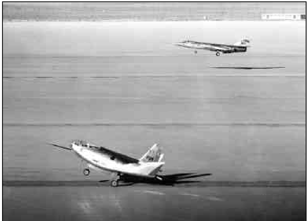
The HL-10 landing on the lakebed with an F-104 chase aircraft. (NASA photo ECN-2367)
