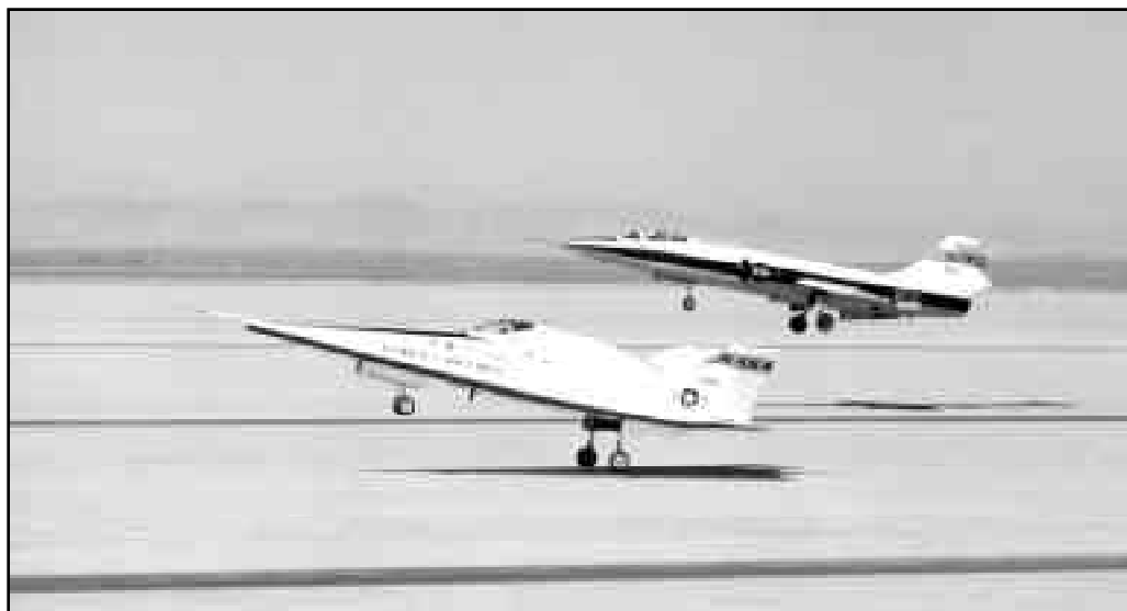
The X-24B landing on the lakebed with an F-104 safety chase aircraft. (NASA photo EC75-4914)
