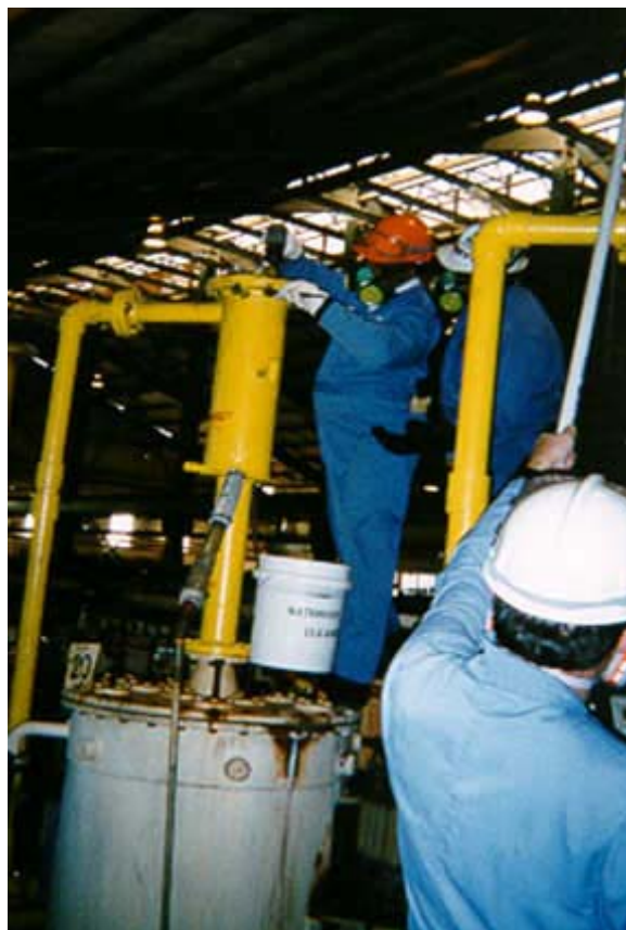
Measuring mercury levels within a chlor-alkali facility (Photo courtesy of Environmental Sciences Division of Oak Ridge National Laboratory, U.S. Department of Energy)
