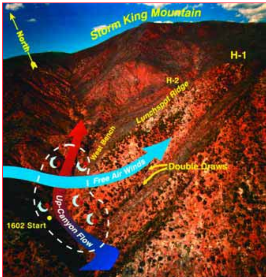
Figure 4—Interaction of the westerly wind flow over the ridgetops burned by the South Canyon Fire and the northerly wind flow up the West Drainage, forming a shear layer (dashed line). The shear layer generated turbulence that helped spread fire and burning embers up the West Drainage and onto the ridgetops. Illustration: USDA Forest Service, Fire Sciences Laboratory, Rocky Mountain Research Station, Missoula, MT, 1998.
