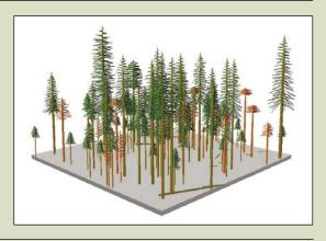
**Ladder-fuel-reduction treatment.** Stands are thinned from below to remove small-diameter trees and underbrush, breaking fuel "ladders" that allow ground fires to move into the crowns. Goals are to reduce ladder fuels, the risk of torching (fire reaching individual tree crowns), and the density of tree crowns so if fire does reach them, it will be unlikely to carry through the whole stand as a crown fire. This example shows a treatment with 80 square feet per acre residual basal area.
