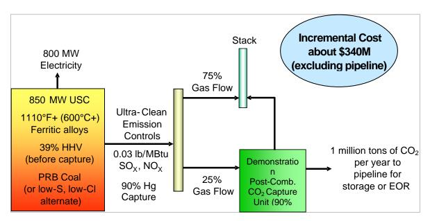
Figure 8 – Key parameters for UltraGen I, assuming a subbituminous feed coal such as Powder River Basin
