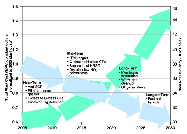
Figure 3 – RD&D path for capital cost reduction (falling arrows) and efficiency improvement (rising arrows) for IGCC power plants with 90% CO<sub>2</sub> capture
