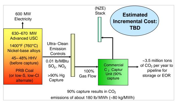
Figure 8 – Key parameters for UltraGen II (upper schematic) and UltraGen III (lower schematic), assuming a subbituminous feed coal such as Powder River Basin
