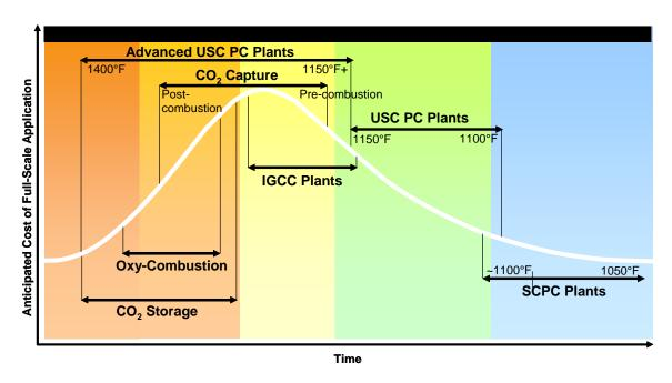
Figure 1 – Model of the development status of major advanced coal and CO<sub>2</sub> capture and storage technologies (temperatures shown for pulverized coal technologies are turbine inlet steam temperatures)
