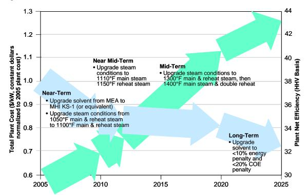
Figure 7 – RD&D path for capital cost reduction (falling arrows) and efficiency improvement (rising arrows) for PC power plants with 90% CO<sub>2</sub> capture
