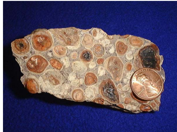
Bauxite ore (pictured) contains small amounts of mercury which can be released into the environment during mining and refining Photo courtesy of USGS
