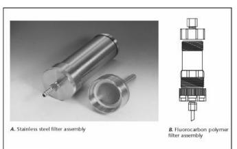
Figure A5-D.1. Apparatus for filtering samples for analysis of dissolved/ suspended organic carbon: (A) stainless steel pressure-filter assembly and (B) fluorocarbon polymer pressure-filter assembly. (Published with permission: A, Gelman Sciences; B, Savillex Corporation.)
