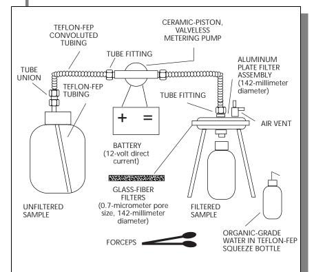
**Figure 5–1.** An equipment system suitable for filtering samples for analysis of organic compounds (from Sandstrom, 1995).
