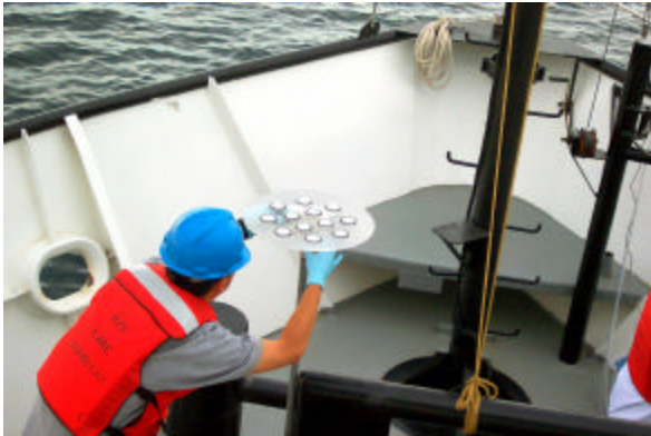
Scientist Puts Out Sampling Plates at the Bow of the R/V Lake Guardian to Collect Dry Atmospheric Deposition (Dust Particles)
