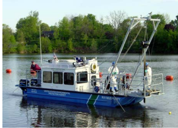
R/V Mudpuppy retrieving sediment core sample
