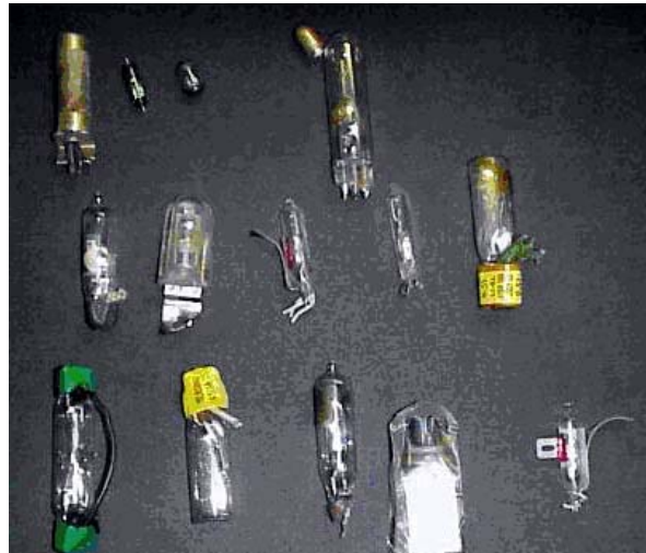
Examples of the types of mercury switches collected (photo courtesy of Wisconsin DNR)
