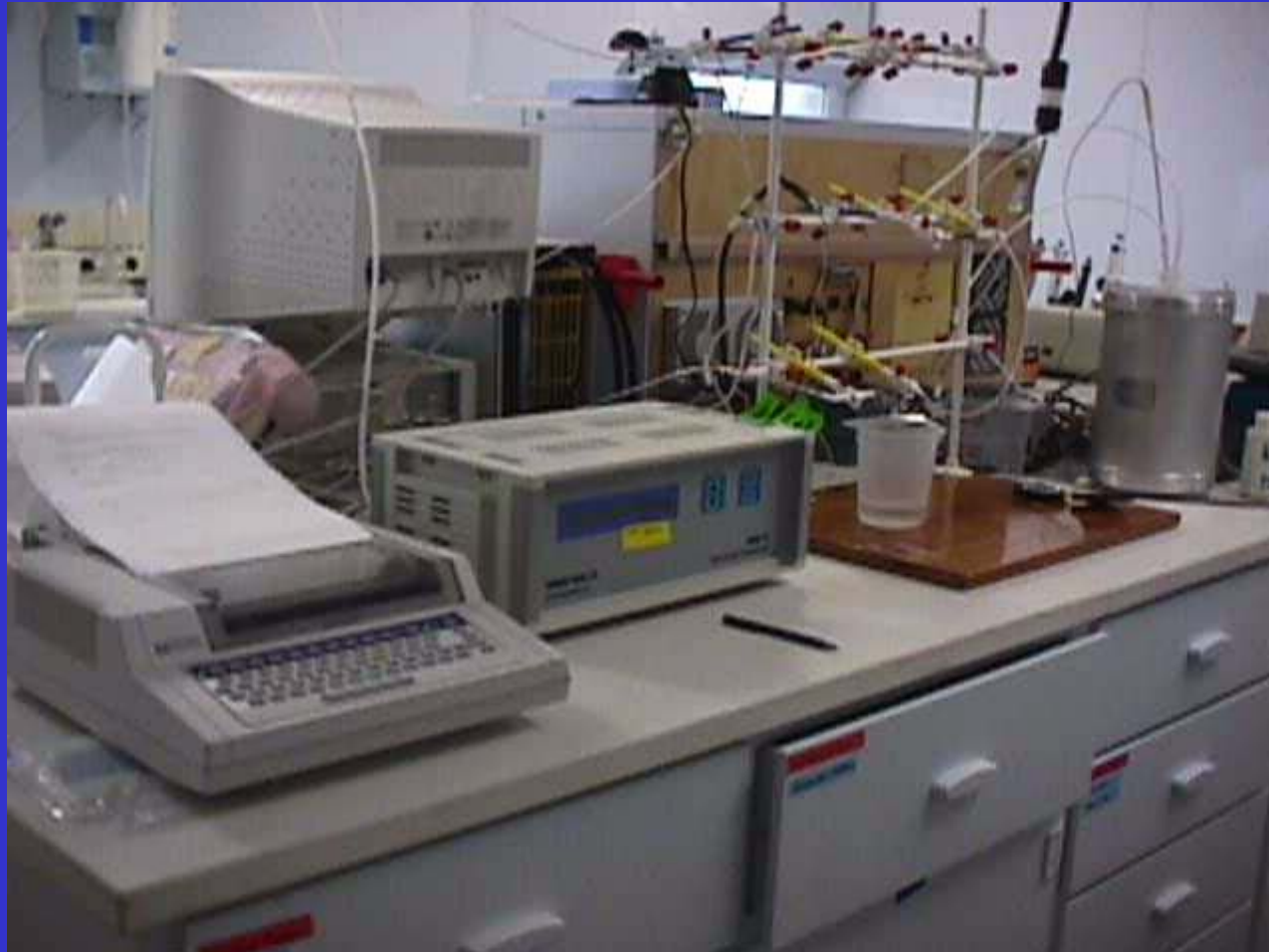
Fig. 15. Photograph of Cold-vapor Atomic Fluorescence Spectroscopy (CVAFS) equipment used for analysis of dissolved-mercury speciation.
