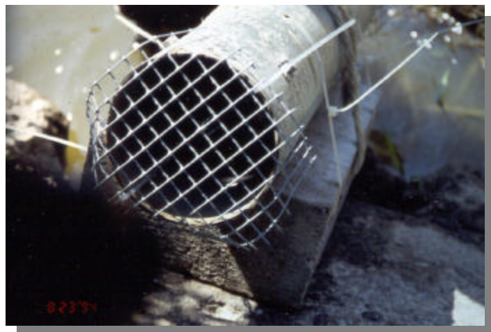
Figure A.7. Modified SPMD deployment device to prevent damage during second deployment period.
