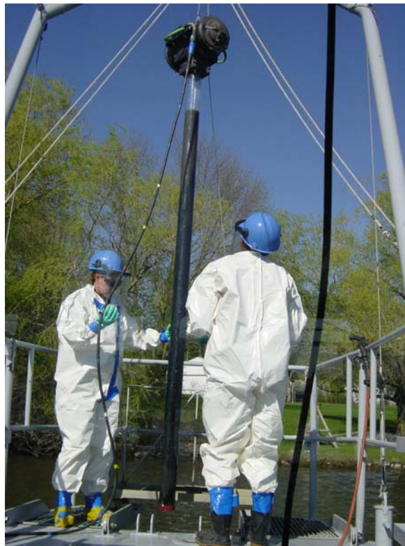
GLNPO Scientists on the R/V Mudpuppy bring up deep sediment core sample
