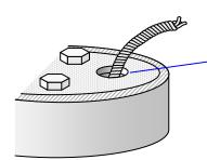
To seal the opening, remove the rope or attach it to an eyebolt on the sanitary seal bottom or drop pipe and use a square-head access plug. For a temporary fix, use silicone seal around the opening.
