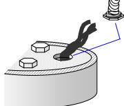
Install an electrical conduit to seal the opening around the wires on a submersible pump. For a temporary fix, use silicone sealer around the opening.
