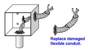
Replace the missing front panel of the electrical box and seal the small holes in the back.
