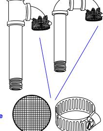
1/2-inch galvanized pipe with non-corrodible 24-mesh screen and a #12 stainless steel adjustable clamp
