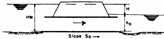
SUBMERGED OUTLET CULVERT FLOWING FULL
