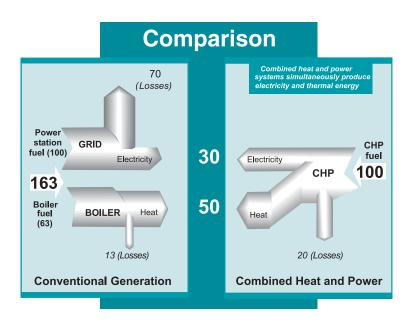
CHP is not a new technology, especially in large industrial facilities. The technologies employed include combustion turbines or smaller reciprocating engines using natural gas or process off gases and waste heat recovery boilers producing steam and power with the exhaust heat from process operations. Recent advances in CHP technologies are steadily reducing the capital costs increasing the efficiencies, and improving the economics of CHP systems.
