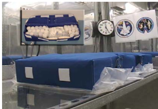
Figure 2. Stability kits inside the Orbital Environmental Simulator at the Kennedy Space Center. Inset shows packages of pills and foods inside the kit (courtesy of L. Putcha).
