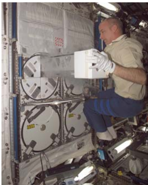
Figure 1. Jeff Williams inserts a sample into the MELFI freezer onboard ISS. One dewar door is open (left) and a tray partially extracted. (ISS013-E-64639).
