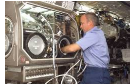
Expedition 13 crewmember Jeff Williams performing the PFMI experiment in the Microgravity Science Glovebox
