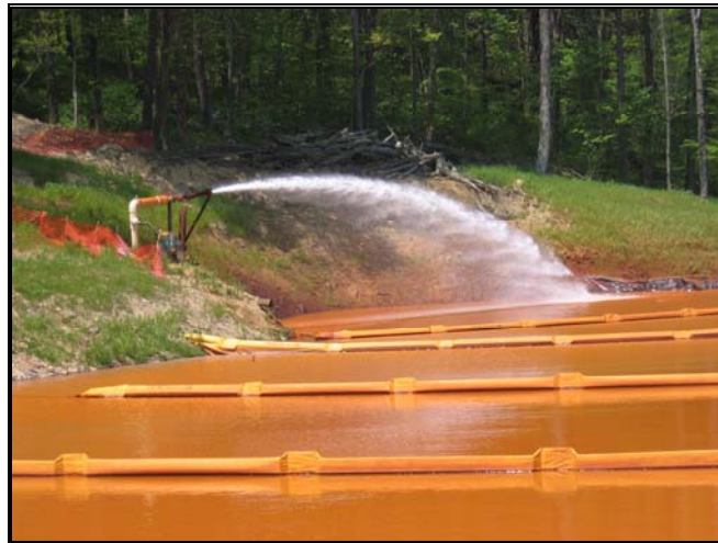
Venturi Aeration Device. Note the immediate iron oxidation.
