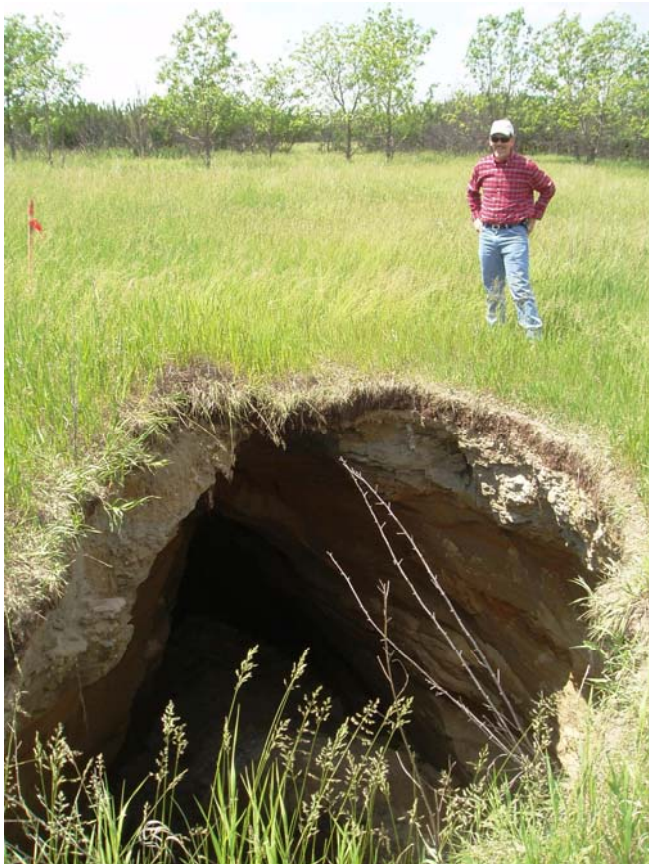
2007 Sinkhole Maintenance Project typical sinkhole scheduled for elimination in vicinity of Beulah, North Dakota
