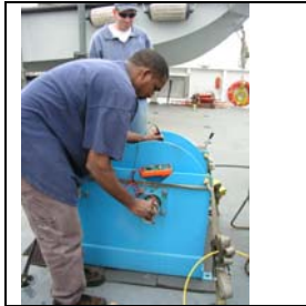
Electrical Engineer working on a grounding system for the winch
