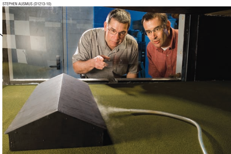
At the National Soil Tilth Laboratory in Ames, Iowa, a low-speed wind tunnel was designed and built to determine the effects of farm buildings and surrounding landscapes on agricultural emissions. Drawing by Jadon Kool.
