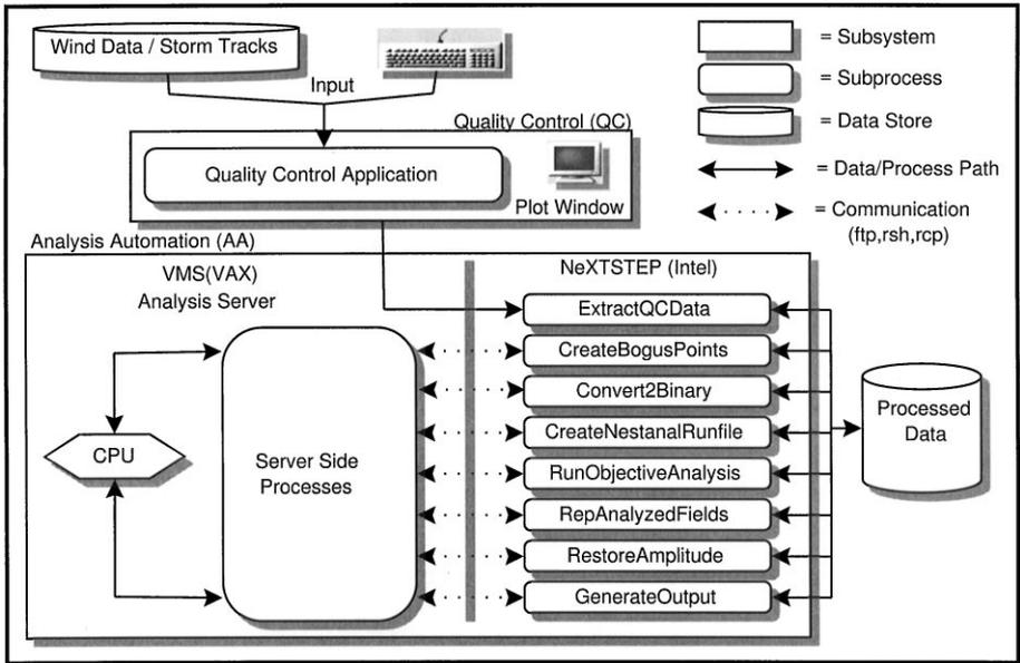
Fig. 2. Process and data flow diagram for WANDA.
