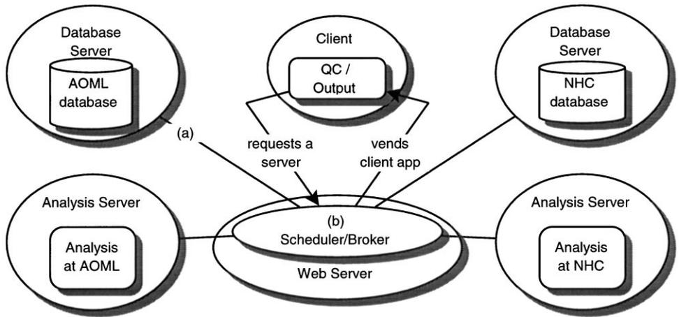
Fig. 9. Future WAnDA application structure. (a) All graph edges indicate possible lines of communication. Directed edges indicate specific actions along those lines. (b) The Scheduler/Broker handles all server requests, vends apps, and manages data flow and load balancing.
