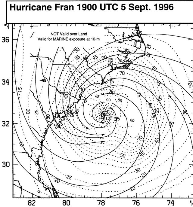
Fig. 6. Real-time analysis sent to NHC. Maximum sustained 1 min surface wind streamlines and Isotachs (kt) using: US Air Force Reserve recon. data adjusted to the surface from 3000 m during 1241–1820 UTC; buoys, drifters, ships, C-MAN from 1600–1800 UTC. 1900 UTC position extrapolated from 1751Z fix using 335° at 14 kts.
