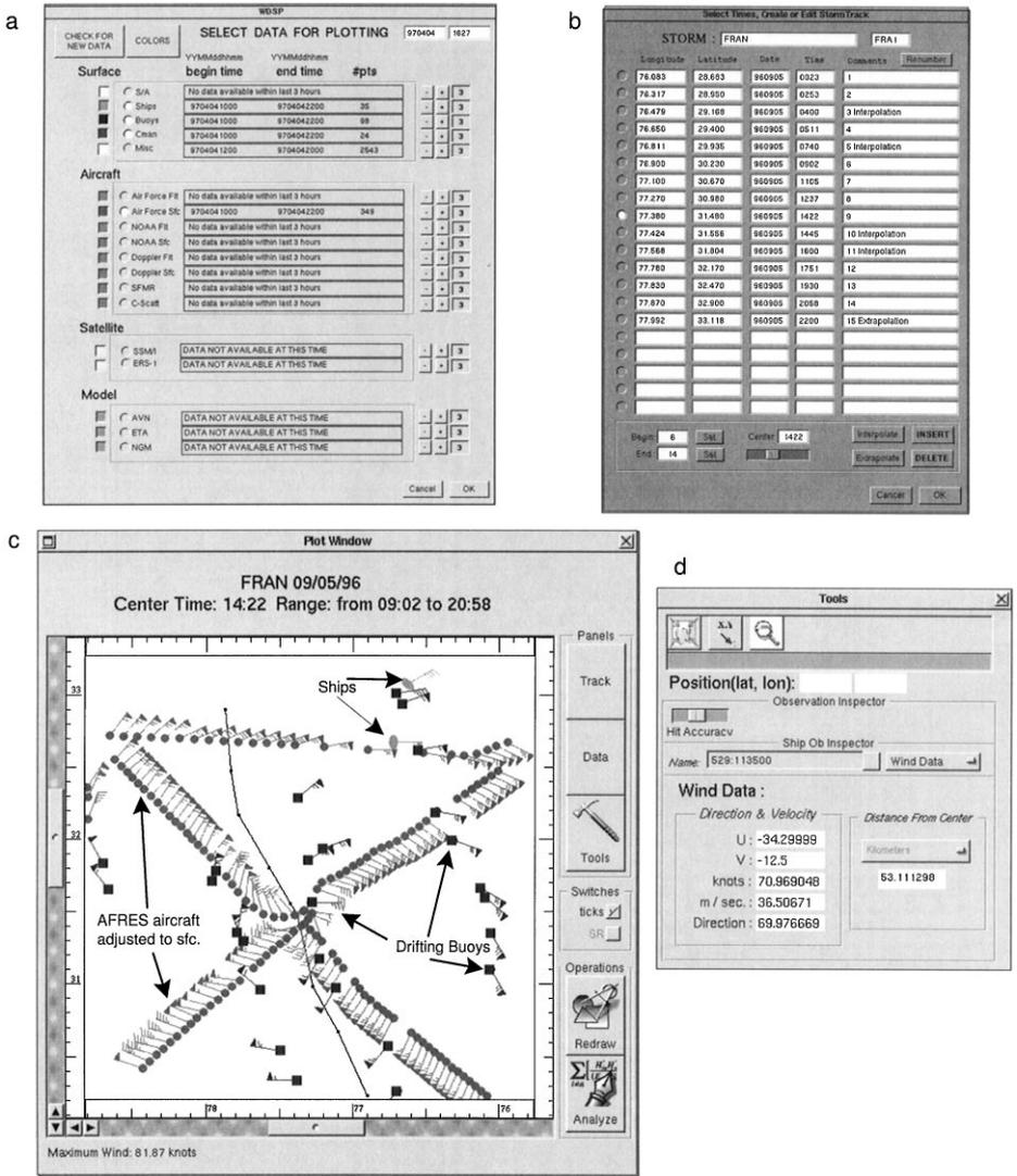
Fig. 3. WANDA user interface elements. (a) Data type selection panel, (b) storm track panel, (c) quality control window displaying Hurricane Fran observations, (d) inspector tool used to examine individual datum.
