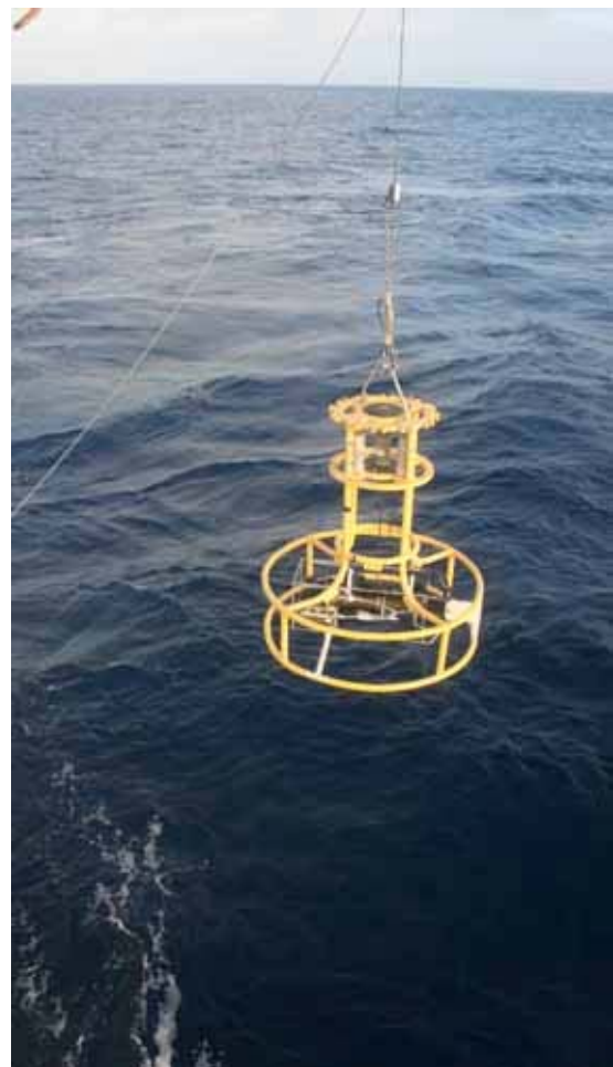
A “rosette” is used to hold the instrumentation for the CTD. Here we see the rosette being lowered down into the water column by way of a crane mounted on the GORDON GUNTER.
