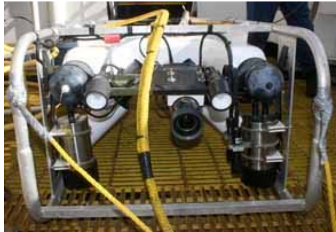
This remotely operated vehicle (ROV) carries both a video camera and a still camera. The yellow umbilical shown in the foreground supplies power and control signals from the GORDON GUNTER.
