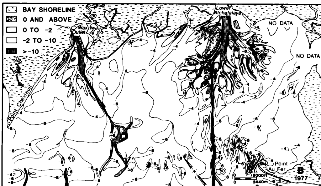
Figure 56. Bathymetric maps of Atchafalaya Bay, (1) 1967 and (B) 1977. Contours are in feet (from Roberts et al. 1980).
