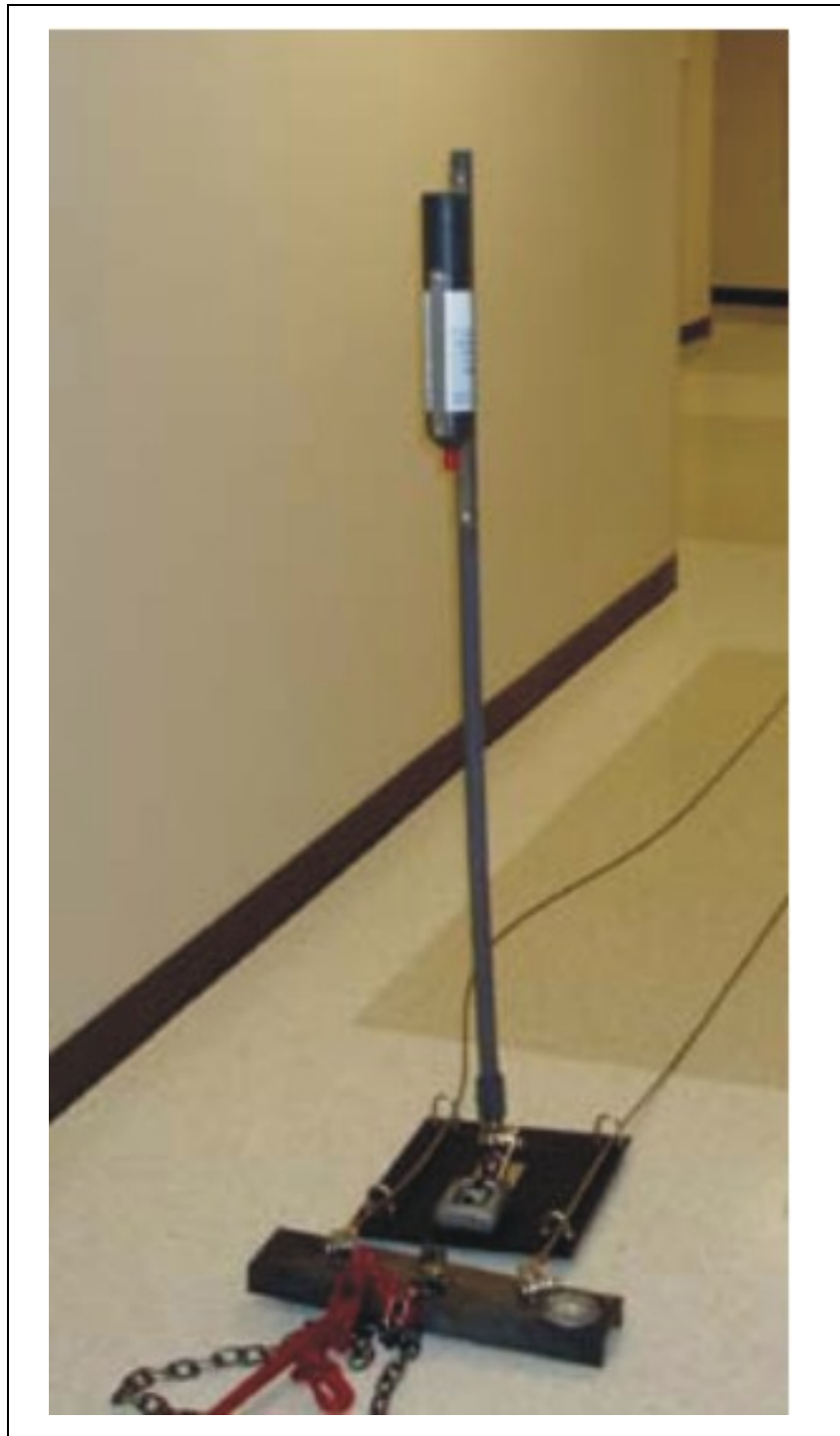
Figure 9. Receiver deployment system including a weighted sled that moved along two guide cables and PVC pipe to which the receiver was bolted, hydrophone end down.
