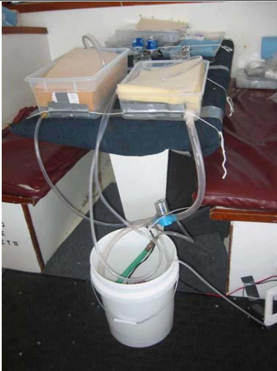
Figure 4. Foam-lined boxes and gill irrigation system used for the surgical procedure.
