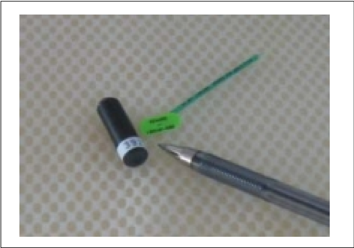
Figure 2. The V8SC-2H acoustic pinger and Floy® internal anchor tag that were implanted into each tagged red snapper.
