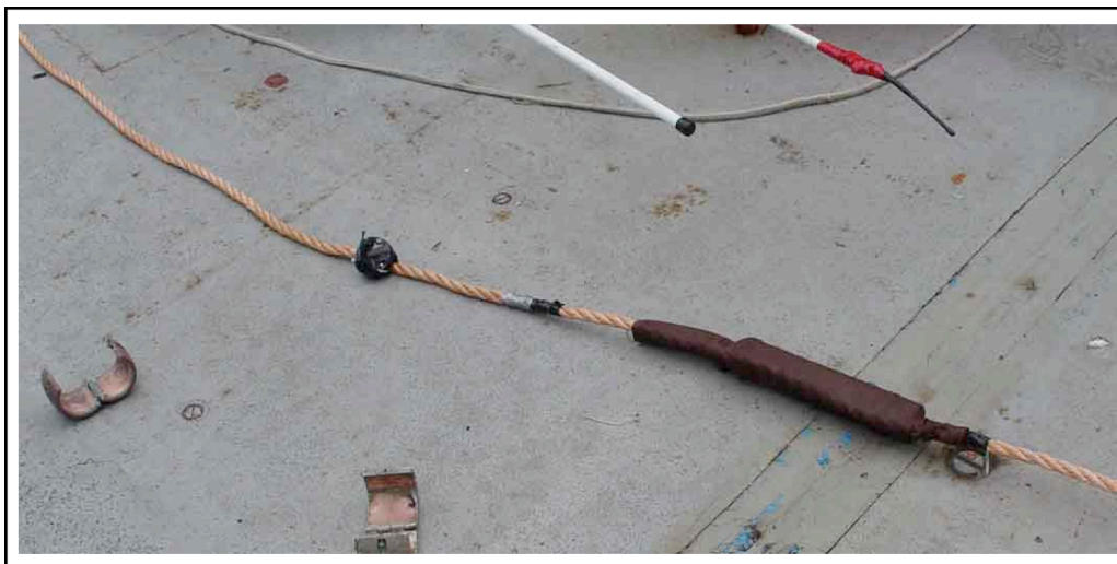
Figure 3.4.2. Flash memory recorder and depth logger attached at the end of a 100-m polypropylene rope. The other end was tied to the end of the SEAMAP array. Note that the hydrophone is taped to the rope as well. This unfortunately led to clipping of the signal.
