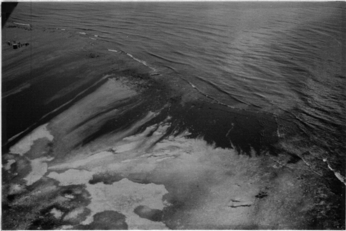
Fig. 4.8 Aerial photograph of oil streaming over the crest of the reef flat at Largo Remo during a rising tide. (The photograph shows approximately 200 m of reef crest extending from upper left to lower right .) During the preceding low tide, winds and waves deposited an accumulation of oil against the seaward side of the reef flat ( right ). The oil moved over the reef crest (from right to left) when the tidal level was high enough to protect the back-reef flat from direct contact with oil slicks.
