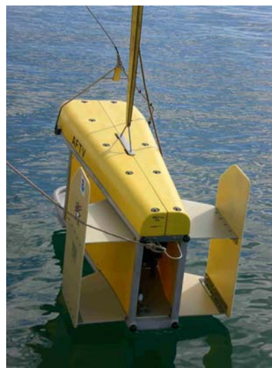
This Advanced Fisheries Towed Vehicle (AFTV) is a recently constructed submersible vehicle that is designed to use acoustical and optical sensors to verify sonar data and evaluate habitat. TAS Jill Carpenter, was present for the initial test launch of the AFTV aboard the DELAWARE II.
