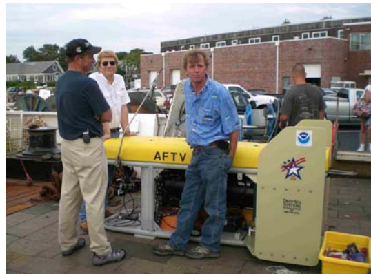
Chief Scientist Bill Michaels (light blue shirt) in front of his new Advanced Fisheries Towing Vehicle (AFTV). This device will be used for the first time when the DELAWARE II completes a hydroacoustic survey. The AFTV uses fiberoptic cables to send real-time images to the ship's computer.
