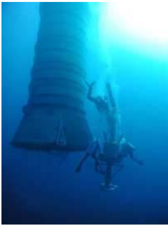
Divers install the equipment need to float the SRB horizontally for towing. The dives can be dangerous, in excess of 130' due to the length of the SRB and up and down wave motion. A decompression chamber is ready on deck.
