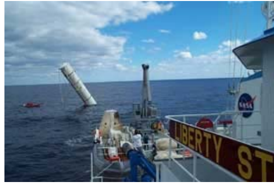
The LIBERTY STAR with SRB and Ambar crew in background and the nose cone already on deck. Winches are used to bring in the parachutes and the crane lifts the nose cone.
