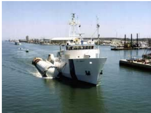
NASA ships M/V LIBERTY STAR and FREEDOM STAR enter port with the SRB's in tow.
