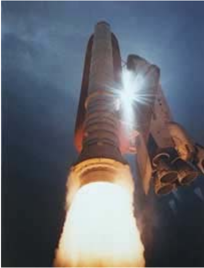
Space Shuttle lifts off from Cape Canaveral. Note the SRB (solid rocket booster), the part where rocket blast is emerging.
