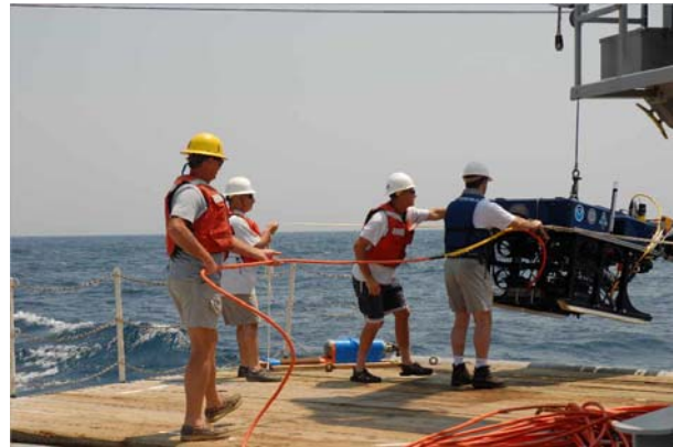
Clockwise: Steve Matthews, Mark Silverman, PJ Zackel, and Andy David use tag lines to control the ROV as it is deployed by the crane.
