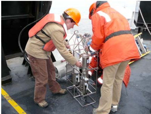
Assistant Survey Technician Stephanie Mills and Physical Scientist Megan Palmer prepare the CTD for deployment.
