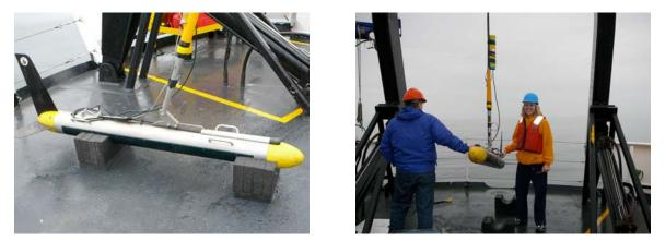
This large torpedo-like device is called a towfish. It is dropped into the water behind the ship to collect pictures of the ocean floor. Teacher at Sea Lisa Kercher assists in bringing it back to deck.
