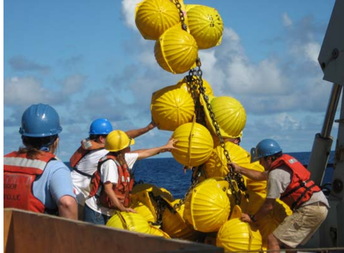
Recovery of mooring floatation on WHOTS-2, consisting of 80 glass balls encased in plastic.
