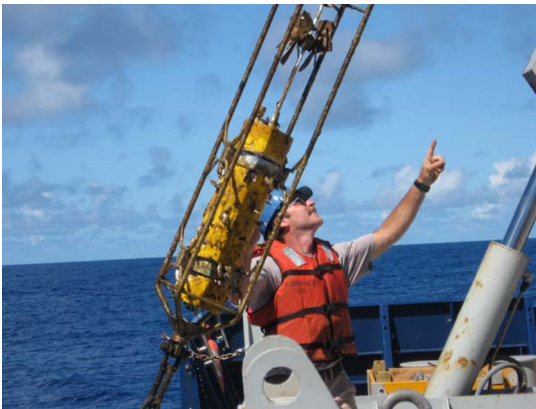
Jeff Lord, engineering technician, directing the recovery of a Vector Measuring Current Meter (VMCM).
