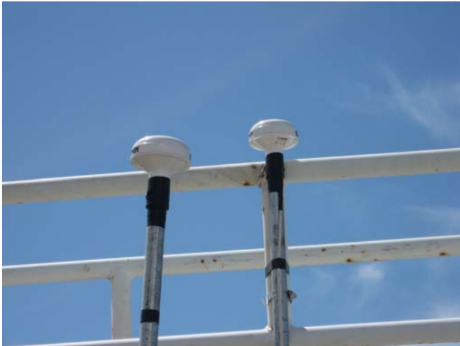
GPS units set up by science team on stern of R/V REVELLE.
