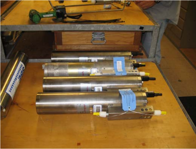
SeaCATs being prepared for mooring.
