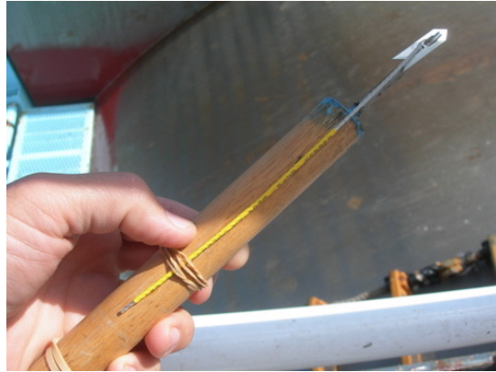
A National Marine Fisheries Service (NMFS) tag and insertion tool.
